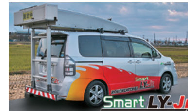
Smart LY-Jr., an Internet-enabled road surface measuring vehicle
